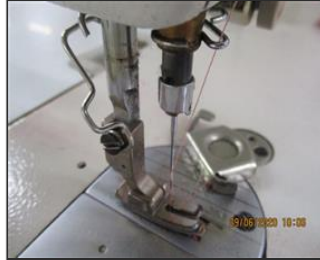
Photo of non-conformity No finger protector device.JPG
