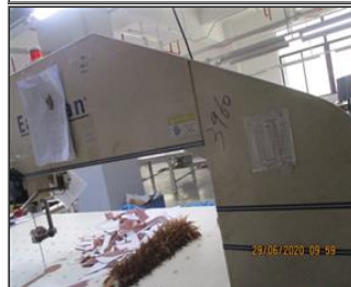
Photo of the personal protection equipments (if applicable) Pulley guard installed for machinery.JPG
